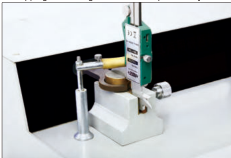
lapping measuring surfaces of caliper lower jaws
