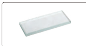
50mm reading scale (check magnification accuracy)
