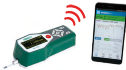
operate roughness tester by mobile phones
