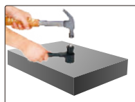
hammer impact to apply test force
